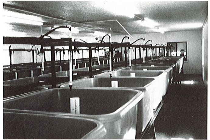
Figure 3. Semi-square tanks used for hatching eggs on mats (Pool Fisheries, Inc., Lonoke).
